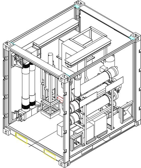
The Outdoor Venture SWRS is a rapidly deployable gray wastewater (used shower and laundry water) reuse system, capable of saving up to 10,000 GPD of potable water demand. The key missions are to serve 150, 300 and 600 man Force Provider and similar military camps with broad use potential.
