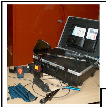
CT-30 kit includes Buster, Lighted Fiber-scope, Radiation Pager, and Probes
