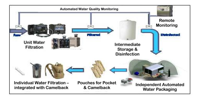
Tactical Integrated Water Purification and Packaging with Remote Quality Monitoring – Avoids Needing Water Specialist in Field Operation
