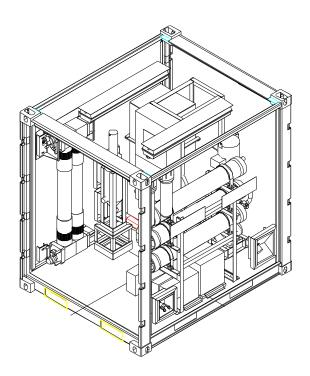
The Outdoor Venture RRWRS is a rapidly deployable gray wastewater (used shower and laundry water) reuse system, capable of saving up to 10,000 GPD of potable water demand. The key missions served are emergency response and disaster relief camps with broad use potential.
